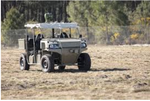
Figure 1: The eRider , developed by SAFRAN, is an all-purpose optionally piloted vehicle that can patrol a given area, observe at long range or carry goods for various off-road applications in difficult environments. These specific vehicles can be either piloted or turned instantaneously into AUGV.
