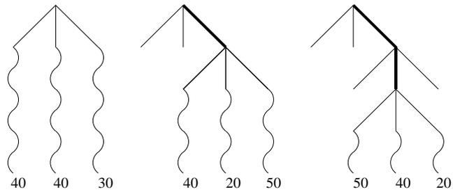
**Fig. 2.** At each step of the principal playout shown here with a bold line, an NMC of level  $n$  performs a NMC of level  $n - 1$  (shown with wavy lines) for each available decision and selects the best one. At level 0, a simple pseudo-random playout is used.
