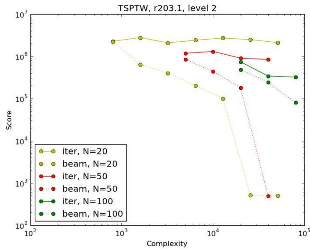
**Fig. 3.** Experience on the problem rc203.1 with level 2. The lower the better. Average on 30 runs. Best results are found by the beam NRPA algorithm with  $N = 20$ . In this experiment, only the beam NRPA algorithm is able to find a valid path, without violated constraints. The best known score for this problem is 453.48. This score is reached for the Beam NRPA with  $N = 20$ .
