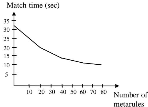
**Fig. 7.** The match time of generated rules decreases when more ordering metarules are generated and used.
