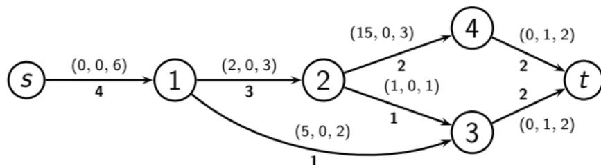
**Figure:** Values on arcs are (cost, lower bound, upper bound). The supply and transportation cost  $C^T(y(\bar{x}^E, \tilde{d})) = 42$ , and the total cost is  $cost(\bar{x}^E, \tilde{d}) = 53$ . The quality of service is  $QoS(\bar{x}^E, \tilde{d}) = \frac{1}{2}(\frac{2}{2} + \frac{2}{3}) = 0.83$ .
