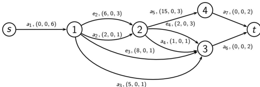
**Figure:** Network  $N$ : values on arcs are  $(c, \text{lower bound}, \text{upper bound})$ .  $I = \{1\}$ ,  $K = \{2\}$ , and  $J = \{3, 4\}$ . The arc set  $A$  is partitioned into original arcs  $O = \{a_1, a_2, a_3, a_4, a_5\}$ , expansion arcs  $E = \{e_2, e_3, e_4\}$ , and demand arcs  $D = \{a_6, a_7\}$ . The demands are  $d_3 = d_4 = 2$ .
