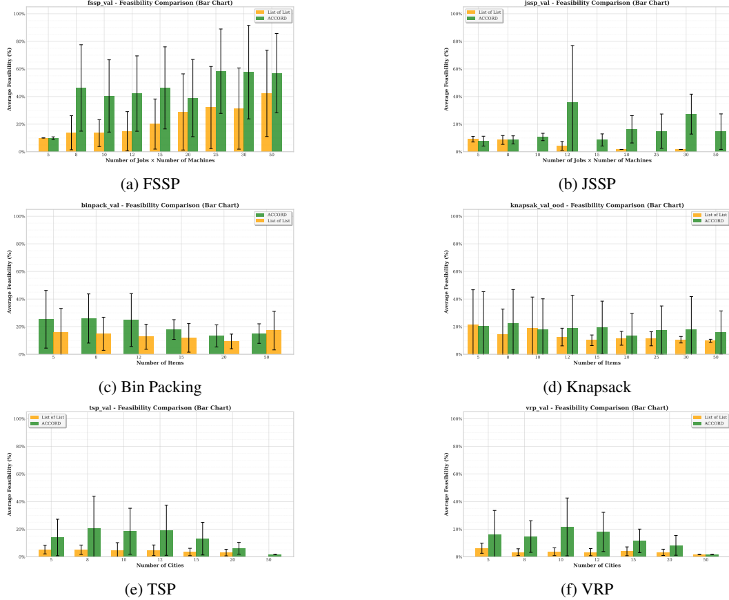
Figure 3: Average feasibility comparison with OR-Tools solution across different problem instance sizes; the higher the feasibility percentage, the better.
