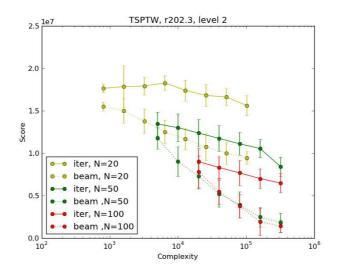
**Fig. 4.** Experience on the problem rc202.3 with level 2. The lower the better. Average on 30 runs. Best results are found by the beam NRPA algorithm with N = 50 and N = 100. The best known score for this problem is 837.72
