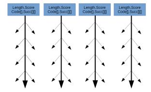
**Fig. 6.** Sketch of information that is stored in a beam of Diversity-NRPA; the buckets on top stand for the beam, thin arrows indicate successors (codes, stored in Succ), the thick arrow the best solution (codes, stored in Code). A duplicate are checked wrt. forks of state and set of successor states.
