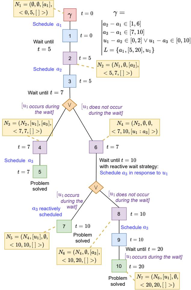
Figure 8: **Detailed R-TDC strategy of a DTNU  $\Gamma$ .** The red square  $\gamma$  is the original DTNU. Other squares are sub-DTNUs, except the  $\nabla$  signs which list transitional possibilities. Nodes  $N_i$  represent the R-TDC strategy nodes as explained in the definition section.
