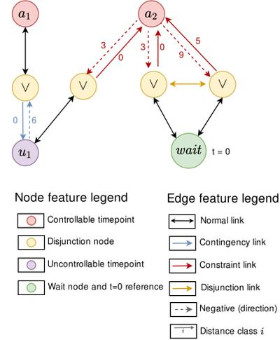
Figure 10: **Conversion of a DTNU  $\gamma$  into a graph.**  $\gamma'$  is the normalized DTNU. Edge distances are expressed as distance classes. To distinguish between lower and upper bounds in intervals, we introduce an additional *negative directional sign* feature.
