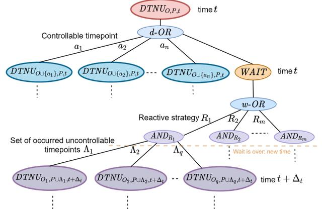
Figure 3: **Structure of the search tree illustrating how a DTNU node is developed.**  $DTNU_{O,P,t}$  (at the root) is a DTNU for which  $O$  is the set of controllable timepoints already scheduled,  $P$  the set of uncontrollable timepoints that have occurred, and  $t$  the time. Each branch  $a_i$  refers to a controllable timepoint  $a_i$ ,  $R_i$  to a reactive strategy for the wait, and  $\Lambda_i$  to a combination of uncontrollable timepoints which can occur during the wait.
