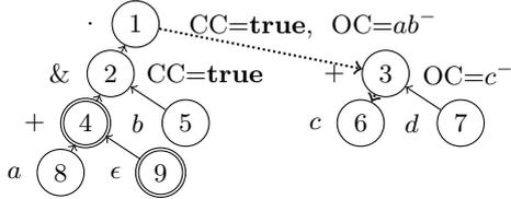
**Figure 7:** The tree for  $T = ((a + \epsilon)\&b[1..5]) \cdot (c + d^+)$  after word  $bbac$  has been read
