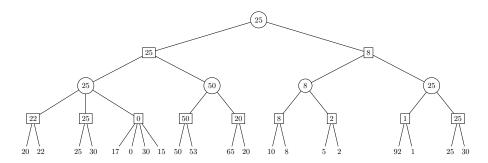
The ALPHA\_BETA algorithm will always return the same value as minimax (i.e. 25). However, it reduces the amount of computation required. The tree below shows some of the procedure involved. The numbers inside the nodes are the returned values for each MAX\_VALUE or MIN\_VALUE (if we are respectively at a max or min node). The numbers on the left side of each node record the values of  $(\alpha, \beta)$  and v at line 5 for each iteration of the 'for' loop in these functions.
