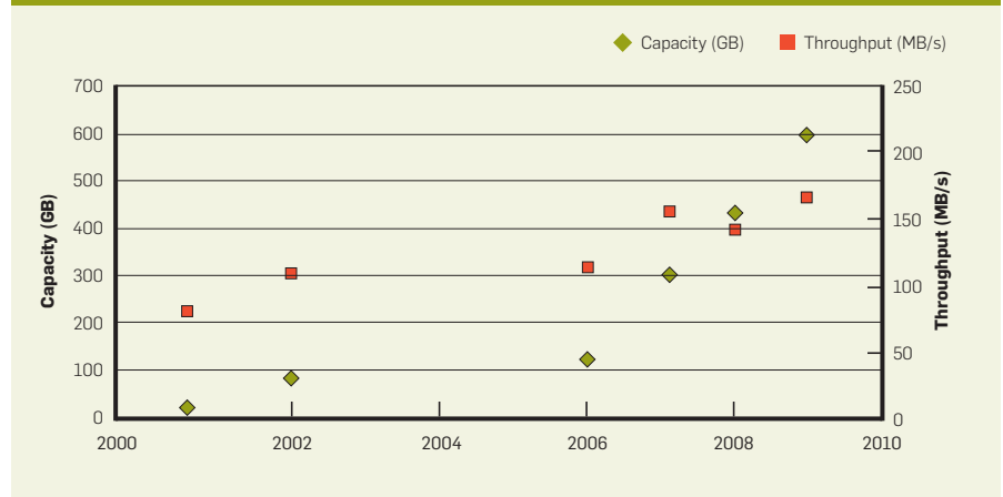
Figure 4. Historical Capacity/Throughput of 15K RPM FC HDDs.
